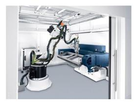
minimum, while the 8KW disk laser combines parts made of almost all materials highly productively. The sensor system "TeachLine" enables exact welding of parts, which leads to a high degree of process stability and production safety.
